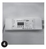
Close terminal block covers and fix with suitable screws. Do not over tighten.
